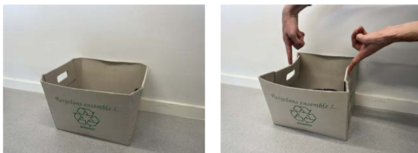
Figure 38: This is an example of a flexible box which is not designed for lifting in compression. (left) Box with out contact. (right) Box after gentle compressive contact. Thus, it would not be well suited for dual arm I.AM. grabbing. Instead it is designed to be held at the handles as a tensile load This type of task requires different end-effectors.
