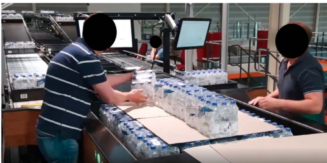
Figure 2: A depalletizing station operated by humans, items are provided one layer at a time and are closely placed together with little to no space in between. Items are picked by the operator and placed on a belt.
